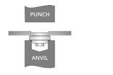
Punch Or Drill Hole To Specified Seat Fastener Squarely In The Hole
